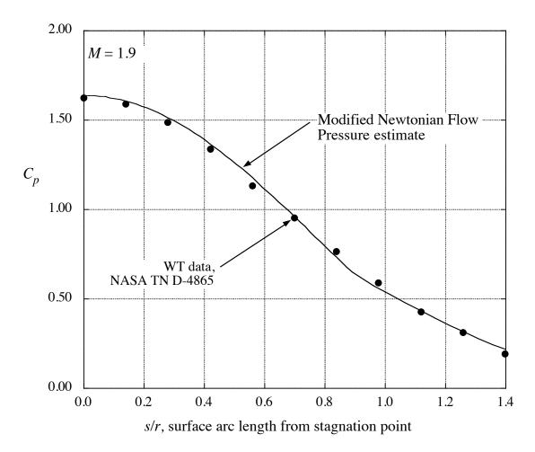
Figure 11-3. Comparison of the modified Newtonian estimate over the nose of a blunted cone with wind tunnel data (Model 2 in TN D-4865).<sup>4</sup>
