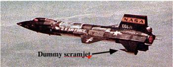
Figure 11-13. X-15 with dummy scramjet (Picture from the NASA Dryden Photo Web Site)
