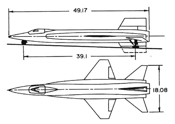
Figure 11-8. Side and top view drawings of the X-15. Note the dashed lines outlining a portion of the ventral tail.<sup>9</sup>
