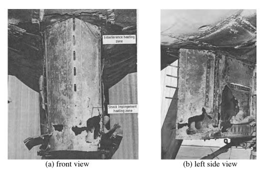
Figure 11-15. The result of aerodynamic heating at M = 6.7 (NASA TM X-1669<sup>18</sup>)
