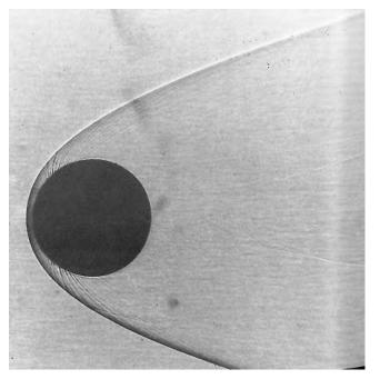
Figure 11-12. Photo of M = 7.6 flow over a sphere (from Van Dyke, *An Album of Fluid Motion*,<sup>14</sup> originally from the Naval Surface Weapons Center).
