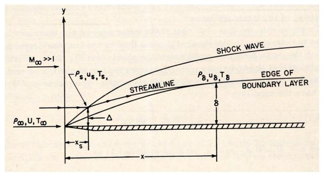
Figure 11-16 Boundary layer development on a flat plate at hypersonic speed.<sup>19</sup>
