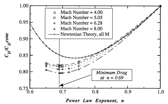
Figure 11-27. Numerical determination of the optimum "n" for power law shapes.<sup>37</sup>
