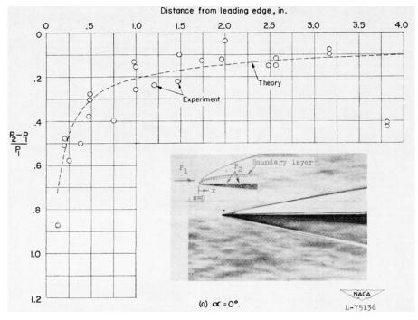
Figure 11-17. Experimental results over a flat plate at zero angle of attack, M = 6.86, Re = 0.98 million from Bertram, NACA TN 2773.<sup>20</sup>
