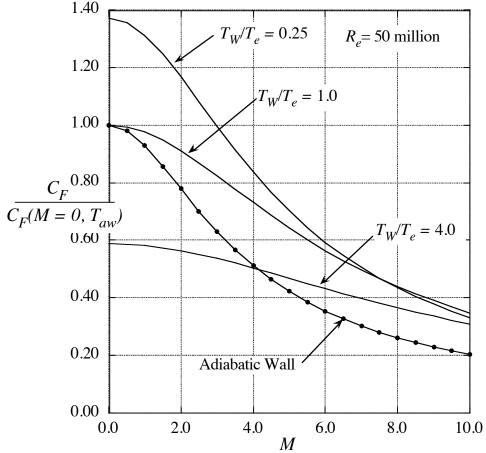
Figure 11-19 Compressibility effects on flat plate skin friction drag coefficient for turbulent flow
