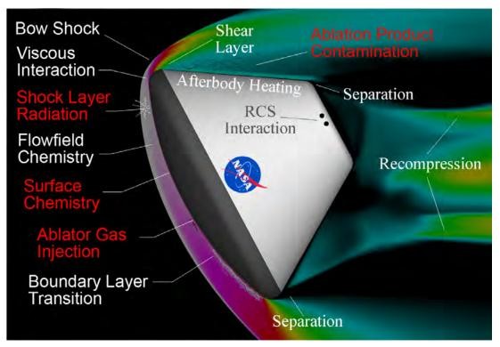
Figure 11-20. The range of gas dynamic consideration required to predict re-entry flowfields.
