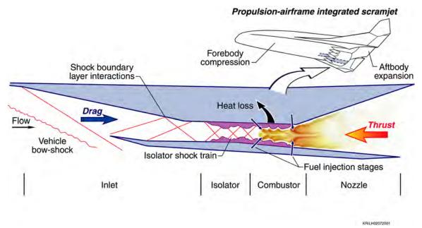
Figure 11-29. Example of engine-airframe integration for a hypersonic aircraft (from Walt Engelund, NASA Langley, May 2001).
