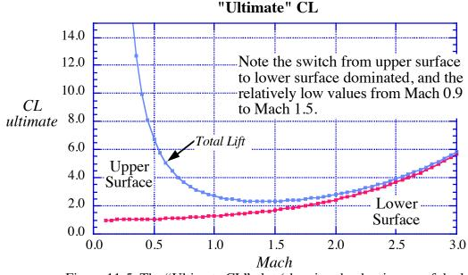
Figure 11-5. The "Ultimate CL" plot (showing the dominance of the lower surface at hypersonic speeds)
