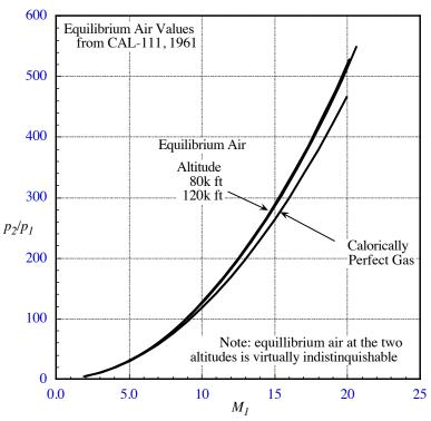
Figure 11-23. Pressure jump across a normal shock wave.
