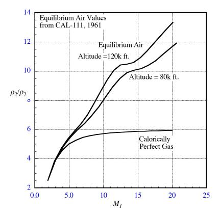
Figure 11-22. Density jump across a normal shock wave.
