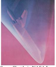
Space Shuttle in NASA Langley Helium Tunnel at M = 20 (NASA SP-440)
