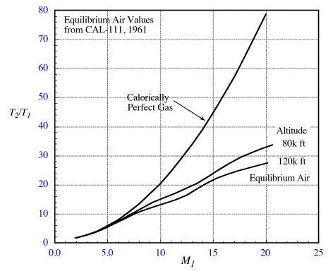
Figure 11-21. Temperature jump across a normal shock wave
