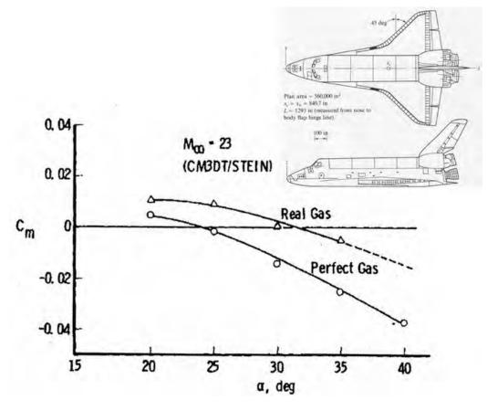
Figure 11-24 Space Shuttle Pitching moment changes with gas model<sup>32</sup> (CM3DT and STEIN are the names of the codes used)
