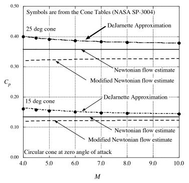
Figure 11-4. Comparison of surface pressures for a cone at zero angle of attack.
