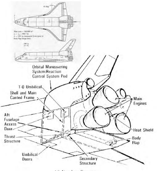
Aft Fuselage Structure
