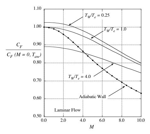
Figure 11-18 Compressibility effects on flat plate skin friction drag coefficient for laminar flow
